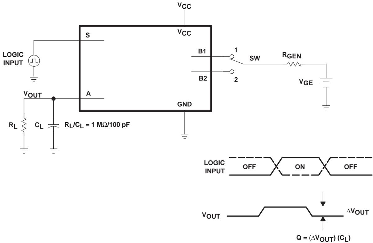
Figure 9. Charge-Injection Test
