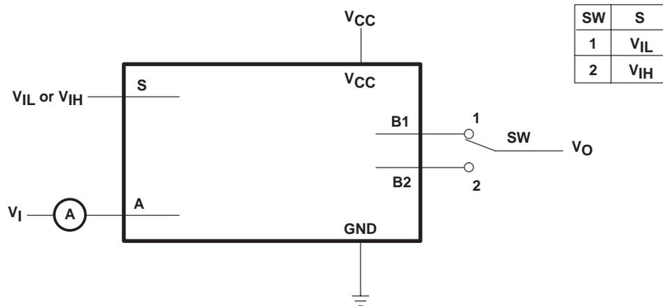
Condition 1:  $V_I = \text{GND}, V_O = V_{CC}$
