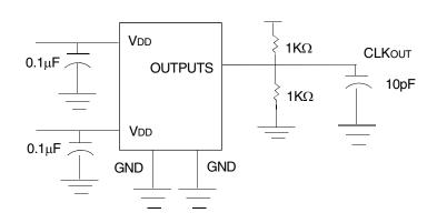
Test Circuit 2 (t8, Output Slew Rate On -1H Devices)
