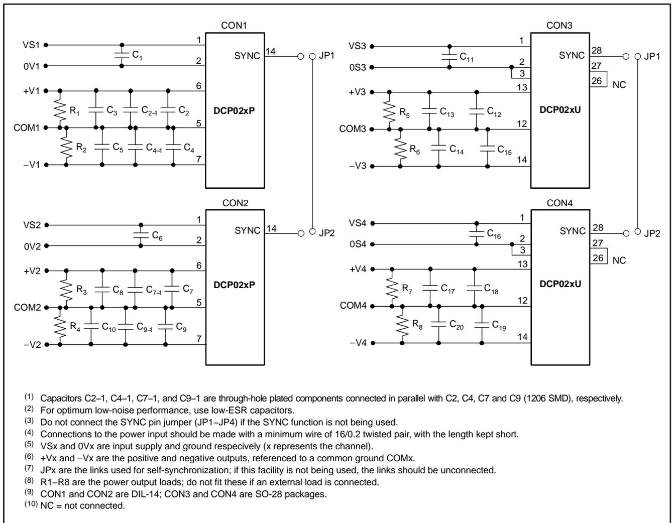
**Figure 7. Example of PCB Layout, Schematic Diagram**
