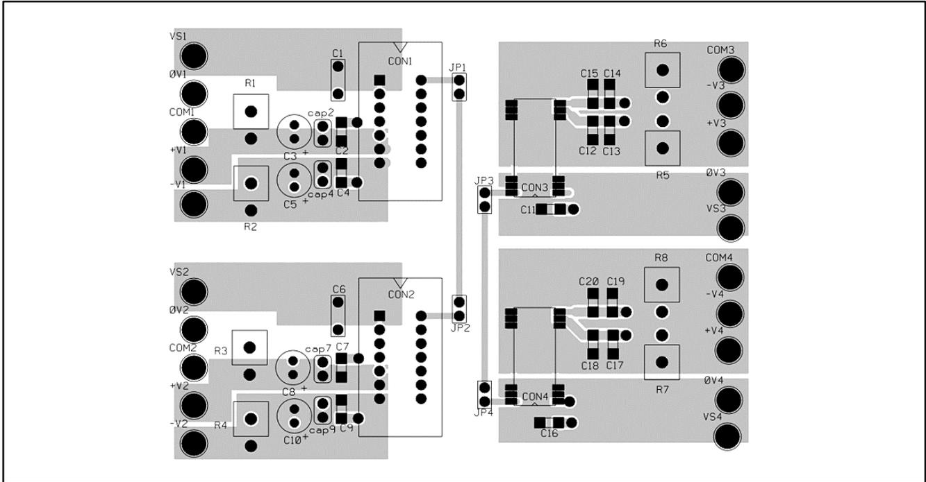
Figure 5. Example of PCB Layout, Component-Side View
