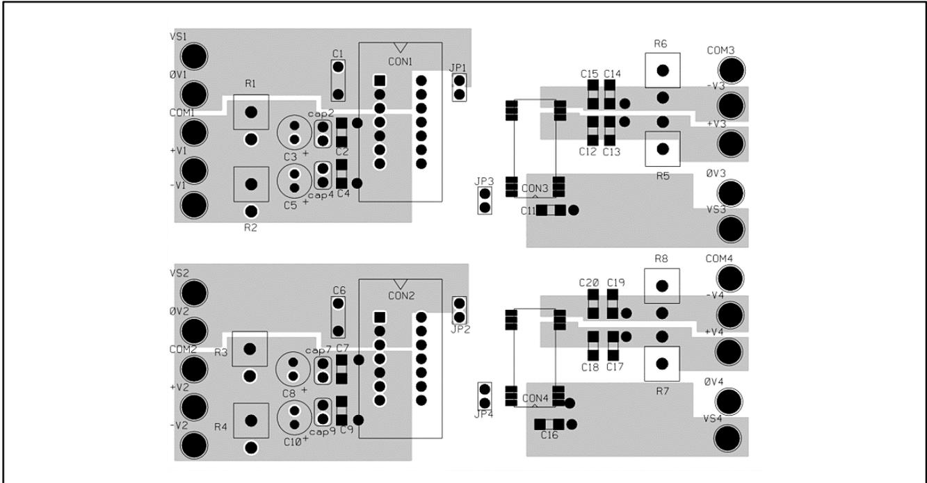
Figure 6. Example of PCB Layout, Non-component-Side View
