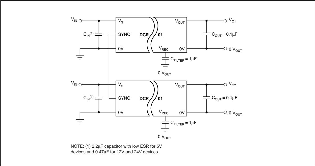
FIGURE 2. Self-Synchronizing DCR01s with a Dual Output.
