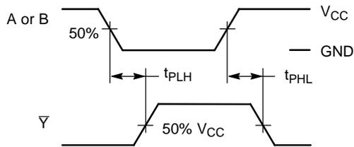
Figure 4. Switching Waveforms
