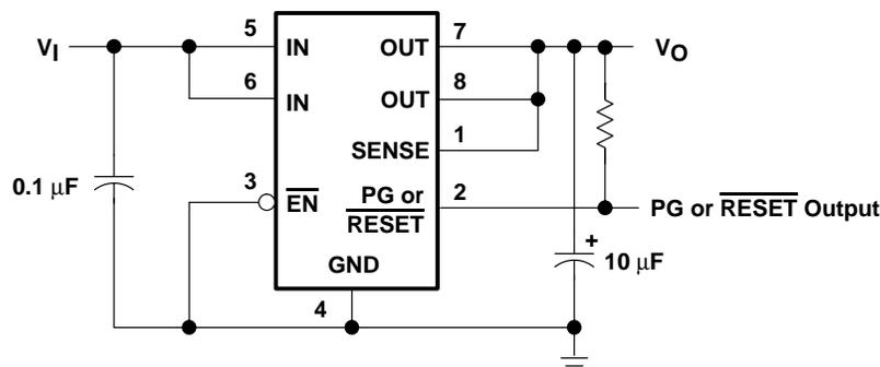
Figure 1. Typical Application Configuration (For Fixed Output Options)
