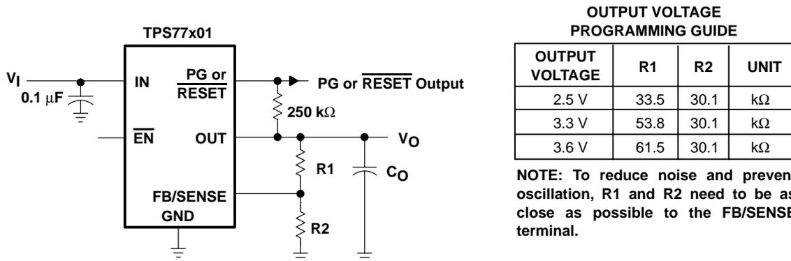
**Figure 24. TPS77x01 Adjustable LDO Regulator Programming**
