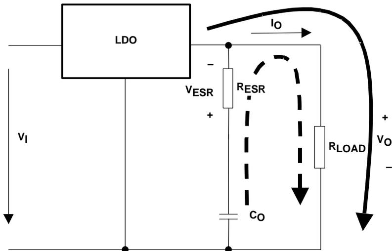
**Figure 22. LDO Output Stage With Parasitic Resistances ESR**
