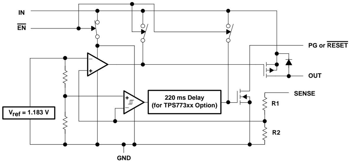
**TPS77301/315/316/318/327/328/333/350 WITH  $\overline{\text{RESET}}$  OUTPUT**
