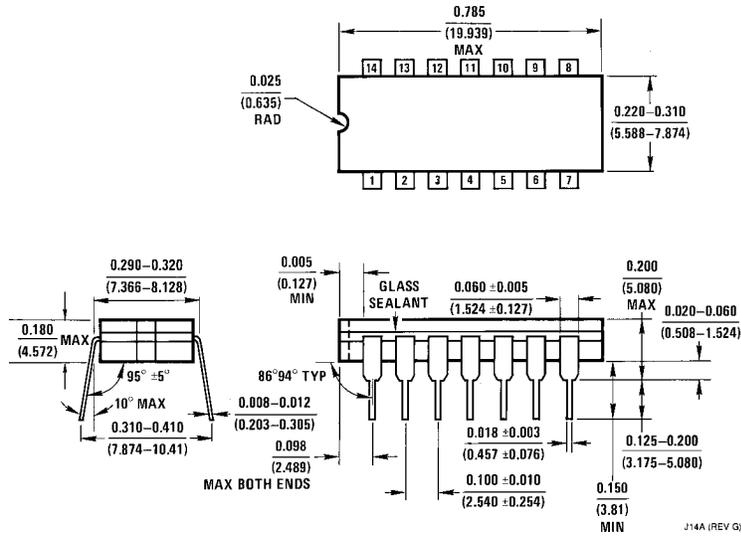
**14-Lead Ceramic Dual-In-Line Package (J)**
