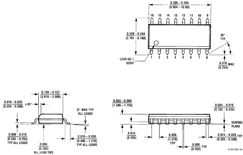
**16-Lead Small Outline Integrated Circuit (SOIC), JEDEC MS-012, 0.150 Narrow
