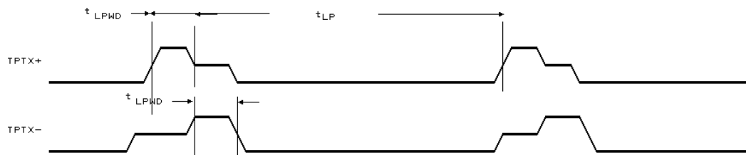
Transmitted Link Integrity Pulse Timing
