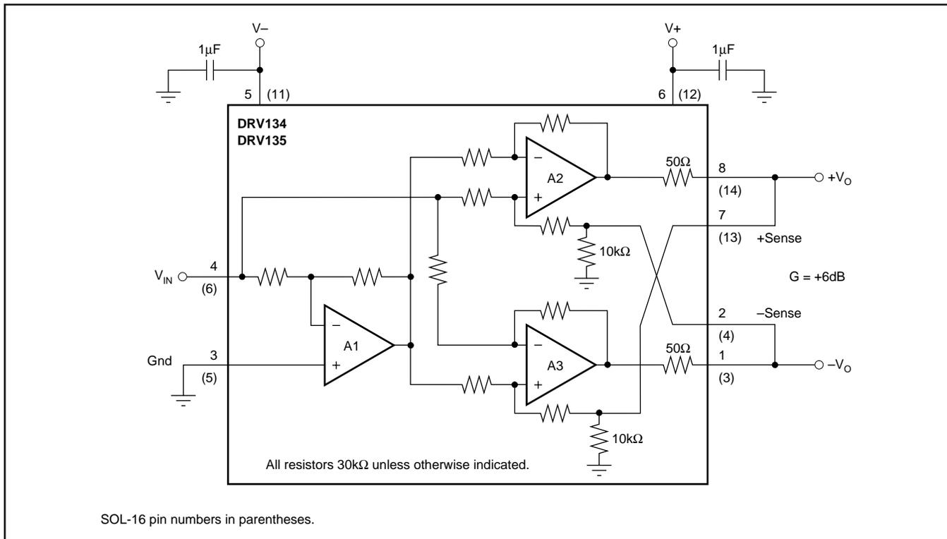
FIGURE 1. Basic Connections.
