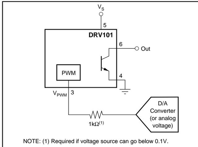
FIGURE 4. Using a Voltage to Program Duty Cycle.
