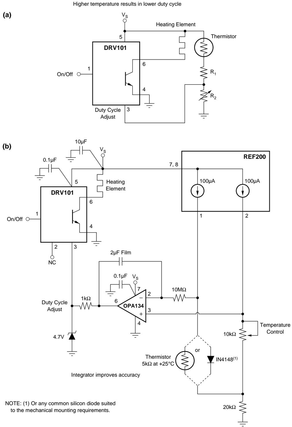
FIGURE 16. Temperature Controller.
