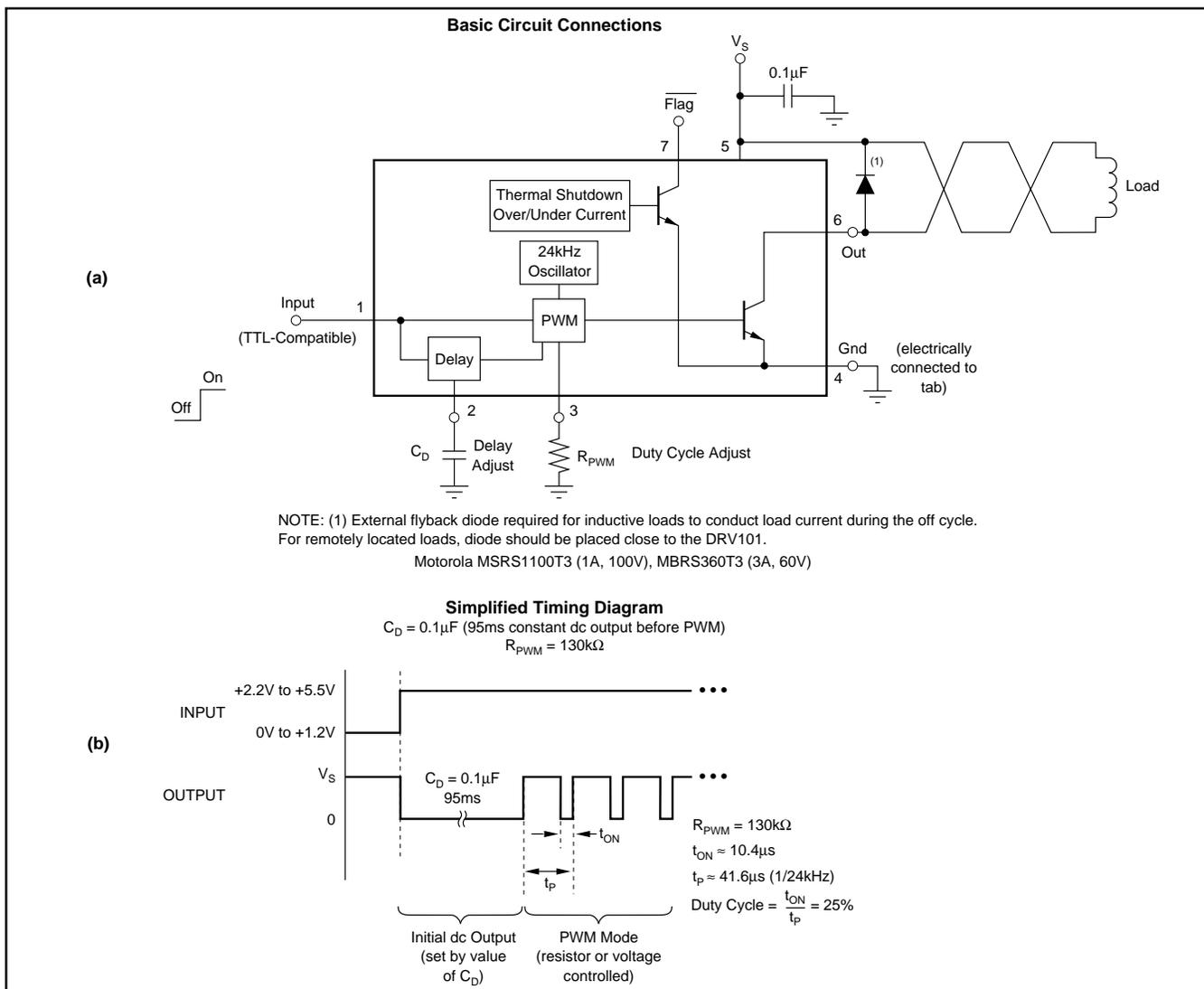
FIGURE 1. Basic Circuit Connections and Timing Diagram.
