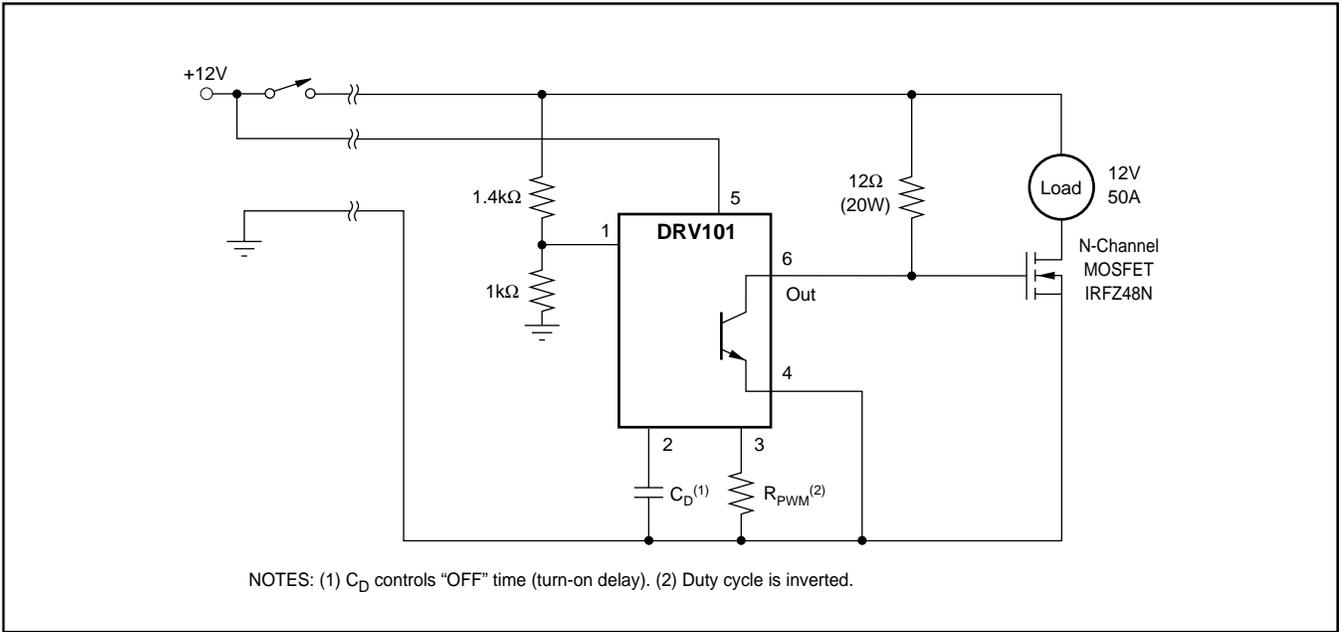
FIGURE 22. High Power, Time Delay, Low-Side Driver.
