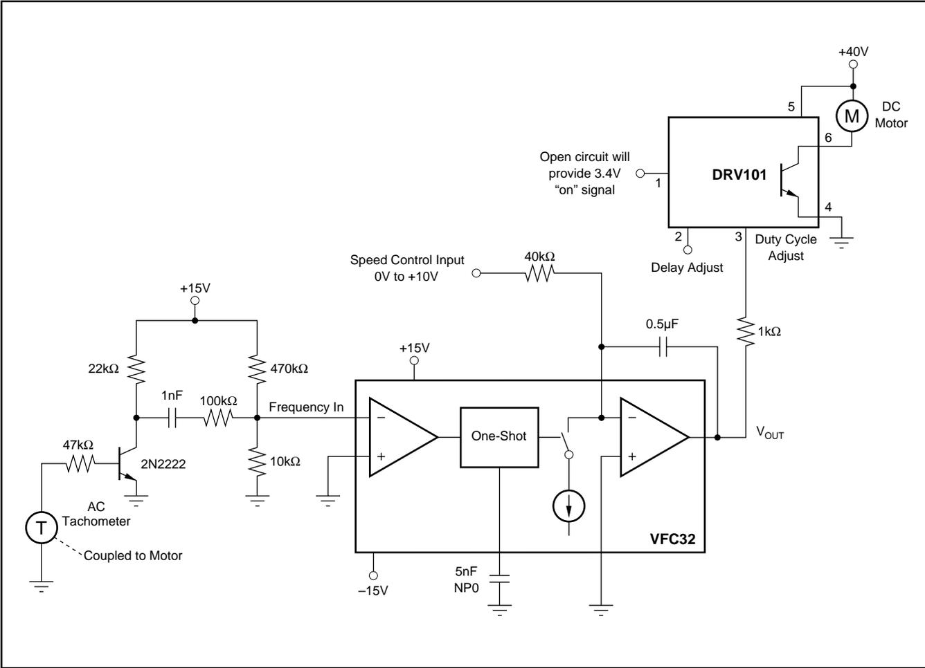
FIGURE 18. DC Motor Speed Control Using AC Tachometer.
