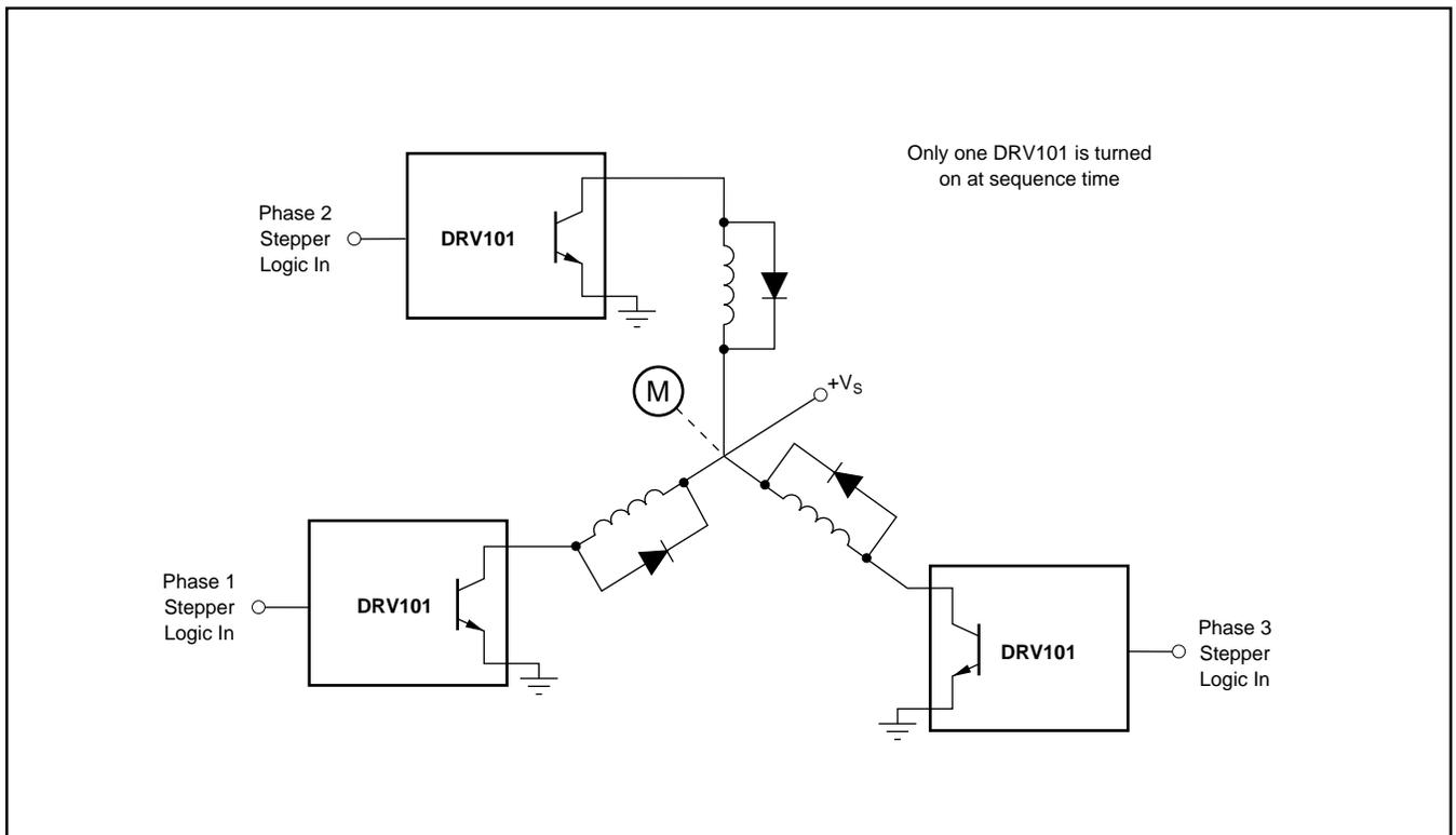
FIGURE 19. Three-Phase Stepper Motor Driver Provides High-Stepping Torque.
