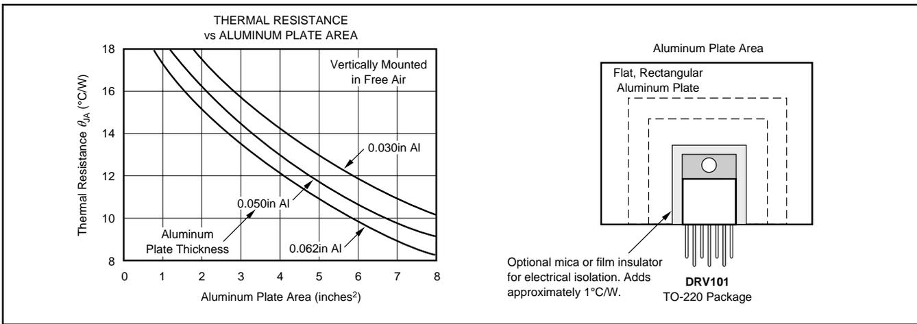
FIGURE 10. TO-220 Thermal Resistance vs Aluminum Plate Area.
