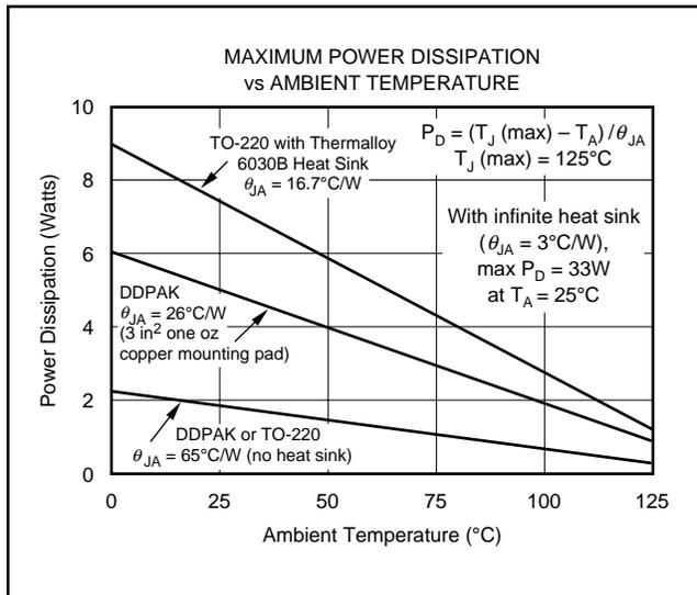
FIGURE 12. Maximum Power Dissipation vs Ambient Temperature.
