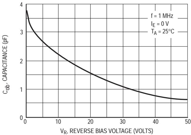
Figure 5. Output Capacitance
