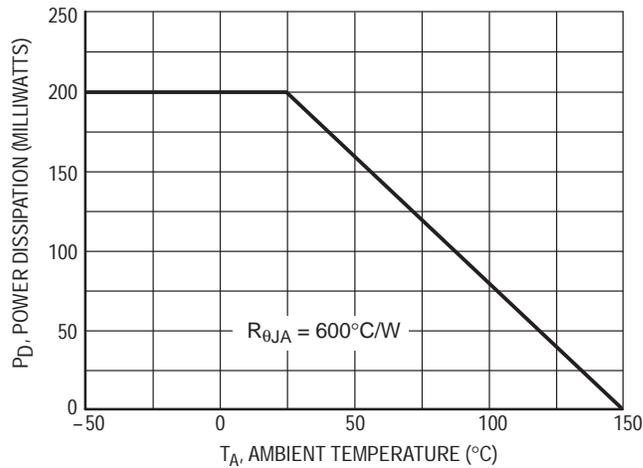
Figure 1. Derating Curve
