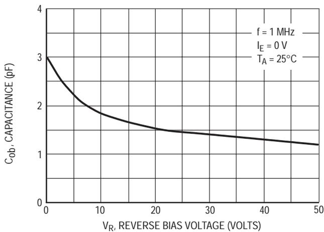
Figure 10. Output Capacitance
