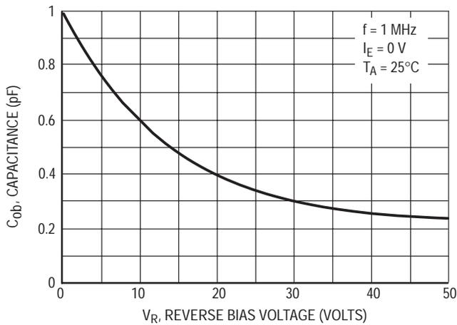
Figure 15. Output Capacitance
