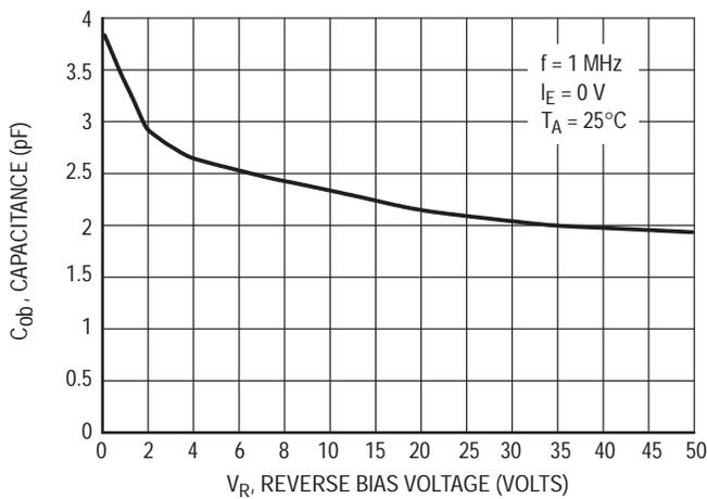
Figure 20. Output Capacitance
