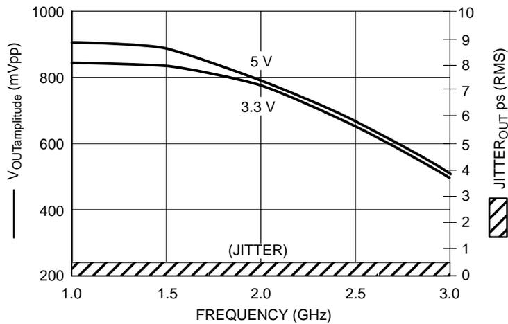
Figure 2. F<sub>max</sub>/Jitter @ 25°C
