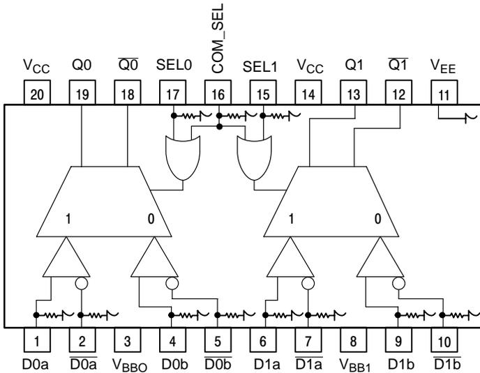
Warning: All  $V_{CC}$  and  $V_{EE}$  pins must be externally connected to Power Supply to guarantee proper operation.
