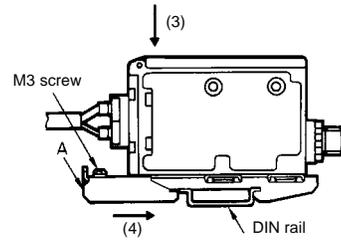
5. Tighten the M3 screw of the E39-L115 to secure the E39-L115.
