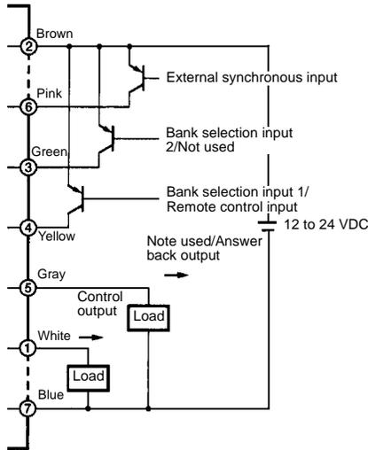
**E3MC-M□41 with PNP Output (4-output Models)**
