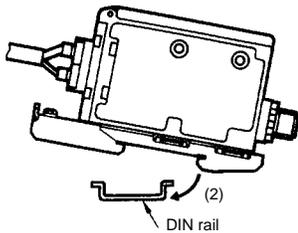
4. Press the E3MC in the direction indicated by arrow (3) and slide part A in the direction indicated by arrow (4) as shown in the following illustration until the E39-L115 correctly engages with the DIN rail.
