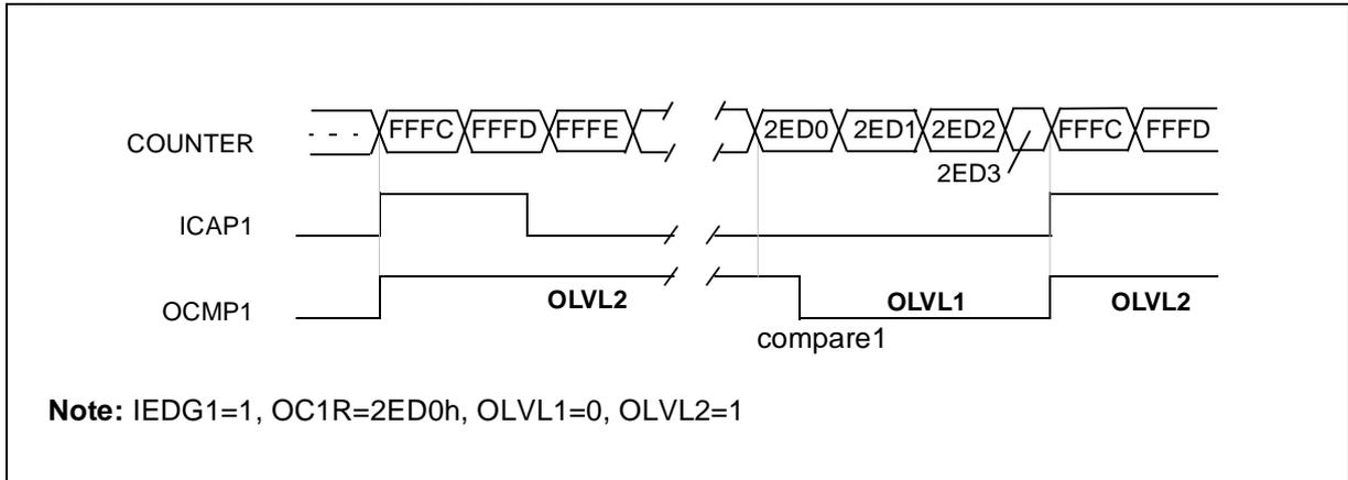
Figure 33. Pulse Width Modulation Mode Timing Example
