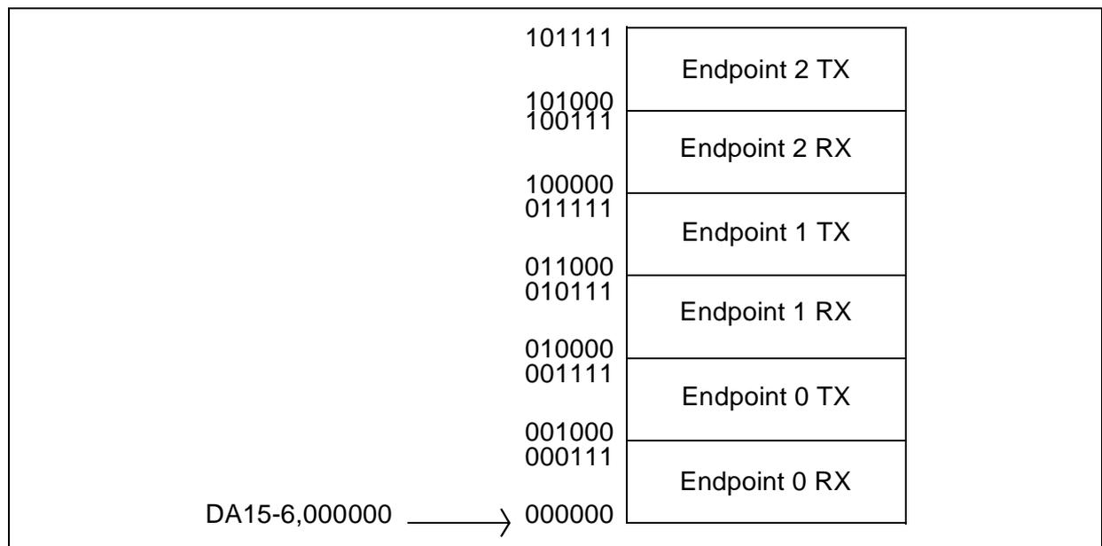
**USB INTERFACE (Cont'd)****PID REGISTER (PIDR)**
