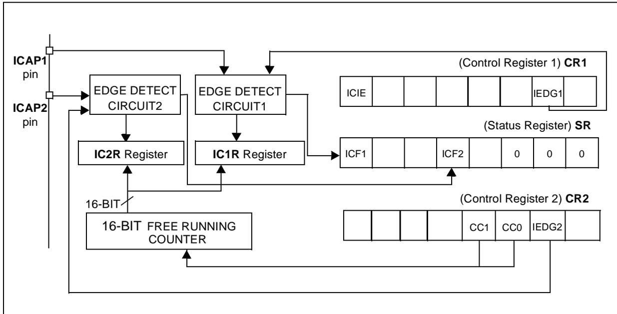
Figure 28. Input Capture Timing Diagram
