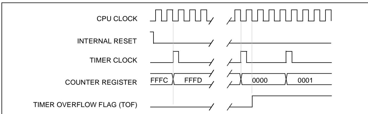
Figure 26. Counter Timing Diagram, internal clock divided by 8
