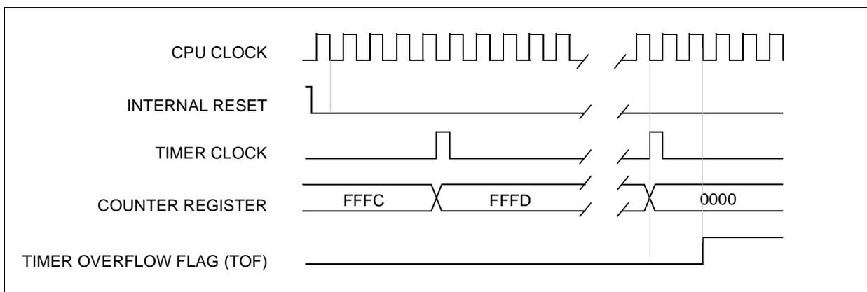
**Note:** The MCU is in reset state when the internal reset signal is high. When it is low, the MCU is running.
