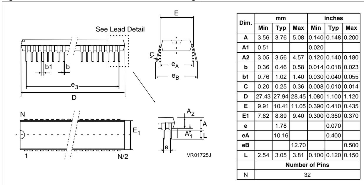
Figure 47. 32-Pin Shrink Ceramic Dual In-Line Package
