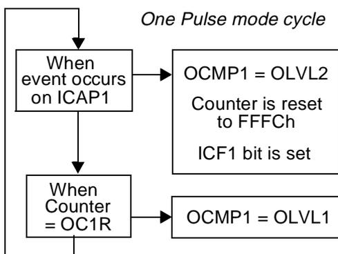
Then, on a valid event on the ICAP1 pin, the counter is initialized to FFFCh and the OLVL2 bit is loaded on the OCMP1 pin, the ICF1 bit is set and the value FFFDh is loaded in the IC1R register.
