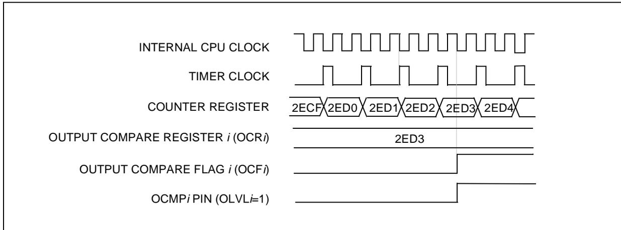
Figure 31. Output Compare Timing Diagram,  $f_{\text{TIMER}} = f_{\text{CPU}}/4$
