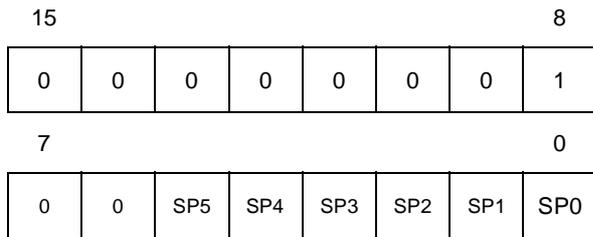
The Stack Pointer is a 16-bit register which is always pointing to the next free location in the stack. It is then decremented after data has been pushed onto the stack and incremented before data is popped from the stack (see Figure 7).
