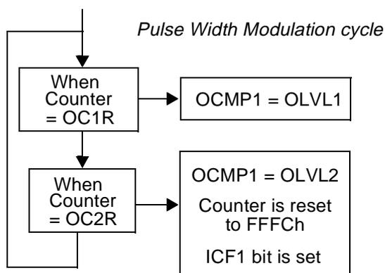
The OC*R* register value required for a specific timing application can be calculated using the following formula:
