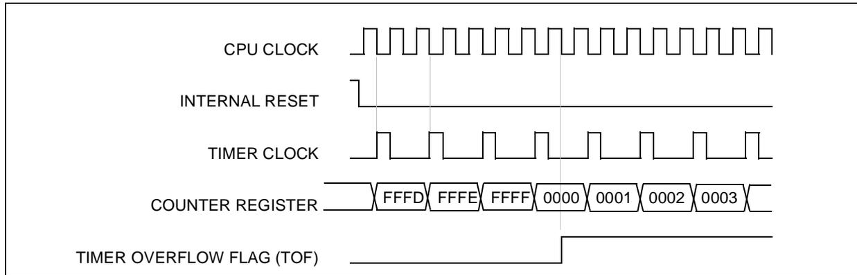
Figure 25. Counter Timing Diagram, internal clock divided by 4
