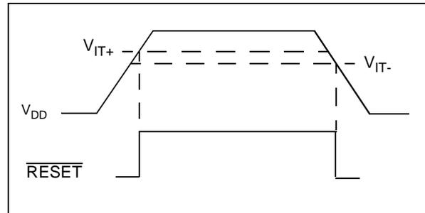
Note: Hysteresis ( $V_{IT+} - V_{IT-} = V_{hys}$ )
