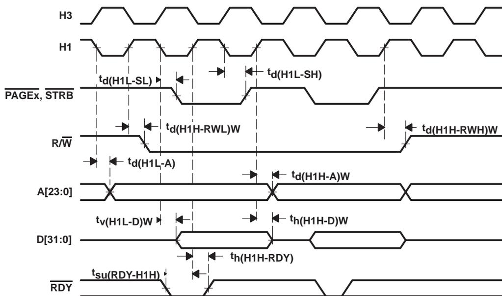
Figure 21. Timing for Memory ( $\overline{STRB} = 0$  and  $\overline{PAGEx} = 0$ ) Write
