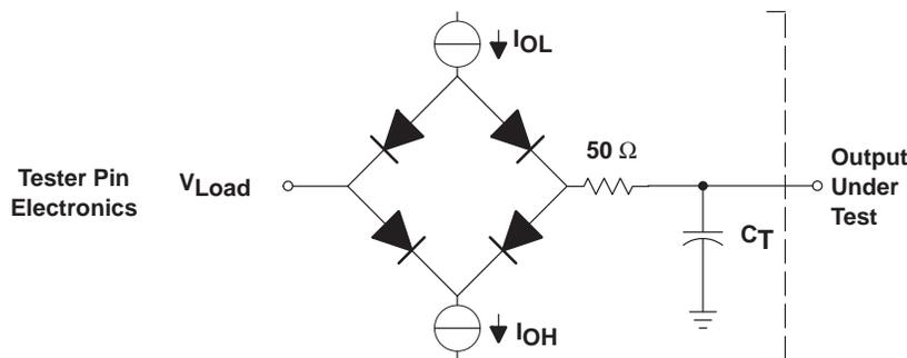
Where: I<sub>OL</sub> = 4 mA (all outputs) for DC levels test.
