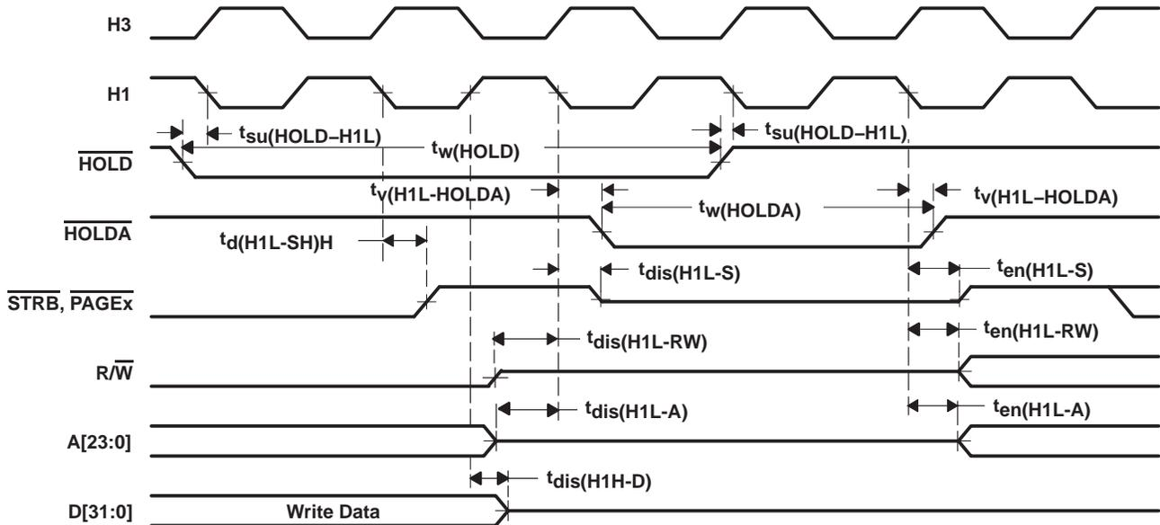
NOTE A:  $\overline{\text{HOLDA}}$  goes low in response to  $\overline{\text{HOLD}}$  going low and continues to remain low until one H1 cycle after  $\overline{\text{HOLD}}$  goes back high.
