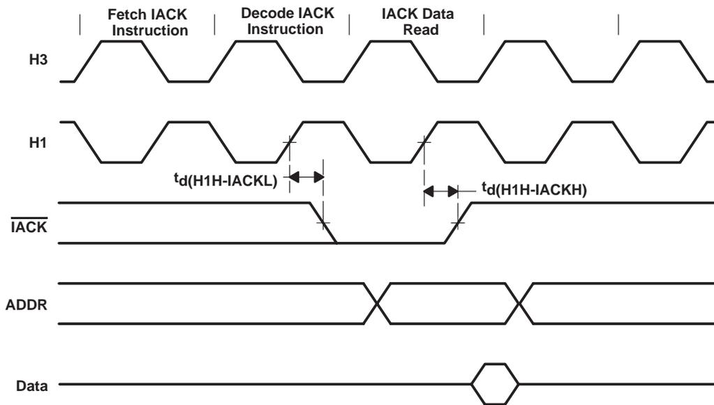
Figure 30. Interrupt Acknowledge ( $\overline{\text{IACK}}$ ) Timing
