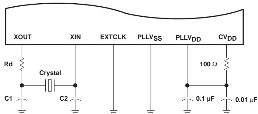
**Figure 5. Self-Oscillation Mode**
