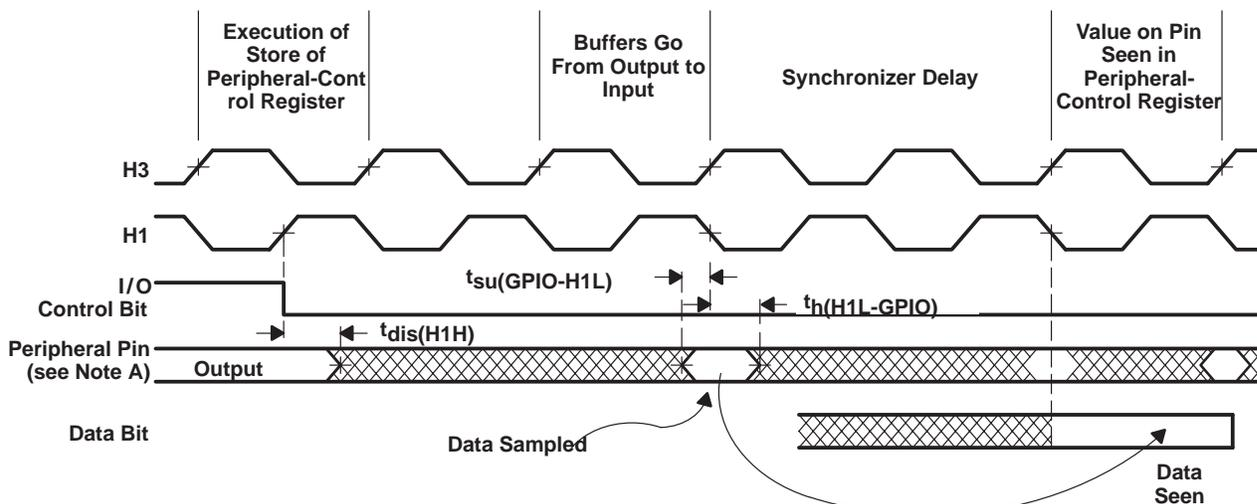
NOTE A: Peripheral pins include CLKX0, CLKR0, DX0, DR0, FSX0, FSR0, and TCLK0/1.
