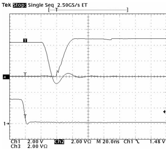
Figure 7. DRVH Fall and DRVL Rise Times
