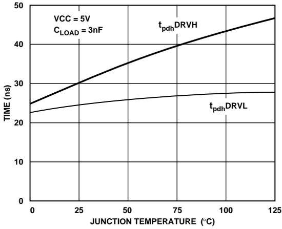
Figure 12. DRVH and DRVL  $t_{pdh}$  vs. Temperature
