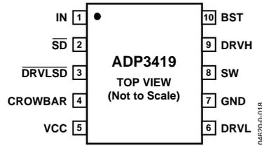
Figure 5. Pin Configuration
