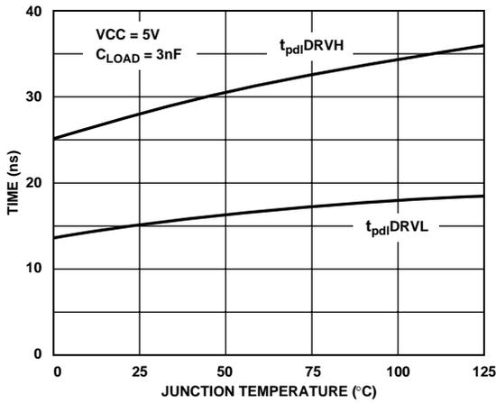
Figure 13. DRVH and DRVL  $t_{pdl}$  vs. Temperature
