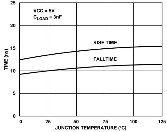
Figure 9. DRVL Rise and Fall Times vs. Temperature
