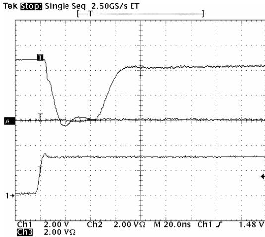
Figure 6. DRVH Rise and DRVL Fall Times
