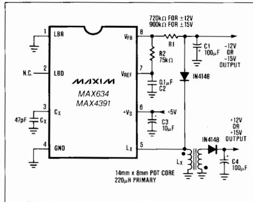
Figure 3. Dual Output, +12V or ±18V DC-DC Converter
