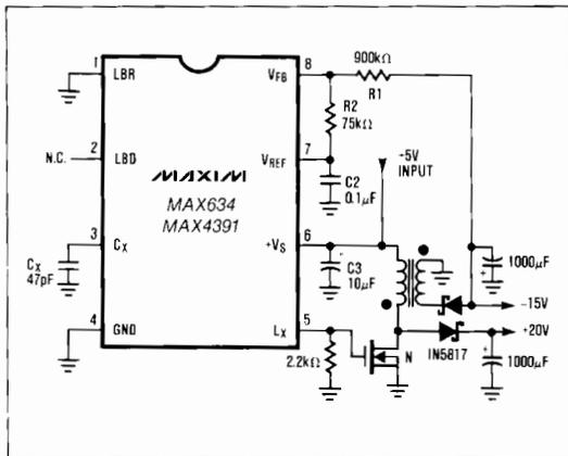
Figure 8. High Power +5V to -15V DC-DC Converter
