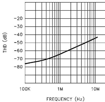
FIGURE 5. DISTORTION vs FREQUENCY
