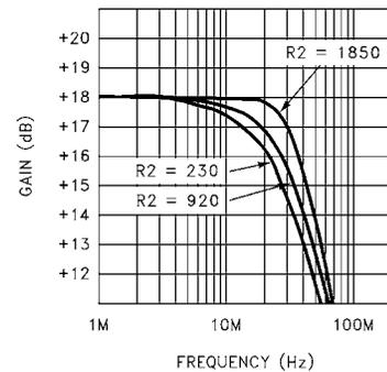
FIGURE 4. FREQUENCY RESPONSE vs RESISTOR R2 (GAIN = 8)
