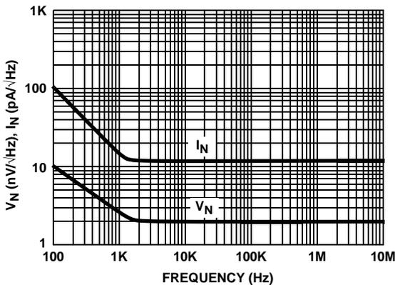
FIGURE 9. VOLTAGE AND CURRENT NOISE vs FREQUENCY
