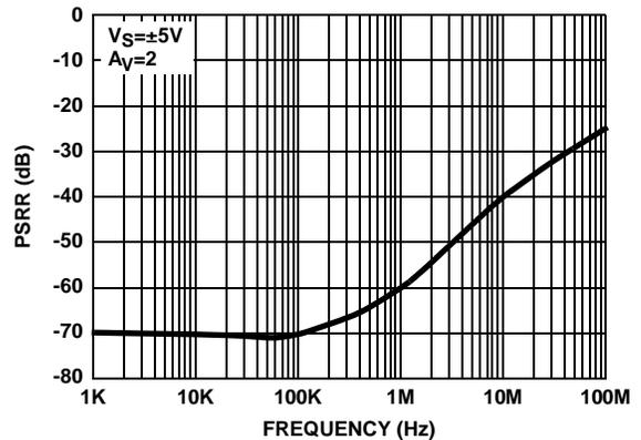
FIGURE 10. POWER SUPPLY REJECTION RATIO vs FREQUENCY
