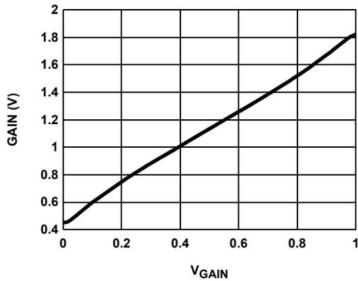
FIGURE 12. VARIATION OF GAIN WITH GAIN CONTROL VOLTAGE
