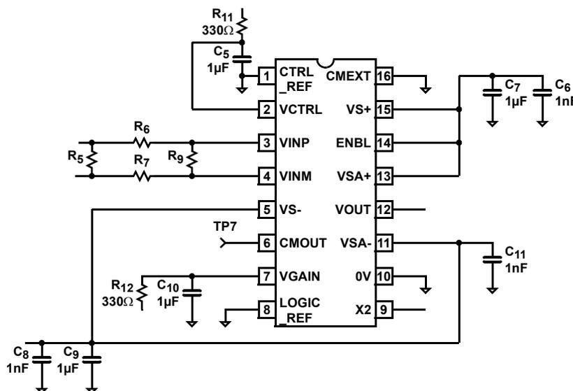
FIGURE 14. CIRCUIT DIAGRAM
