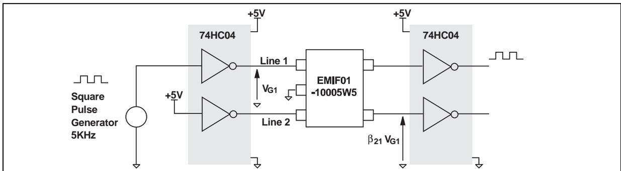
Figure A8 shows the measurement circuit used to quantify the crosstalk effect in a classical digital application.
