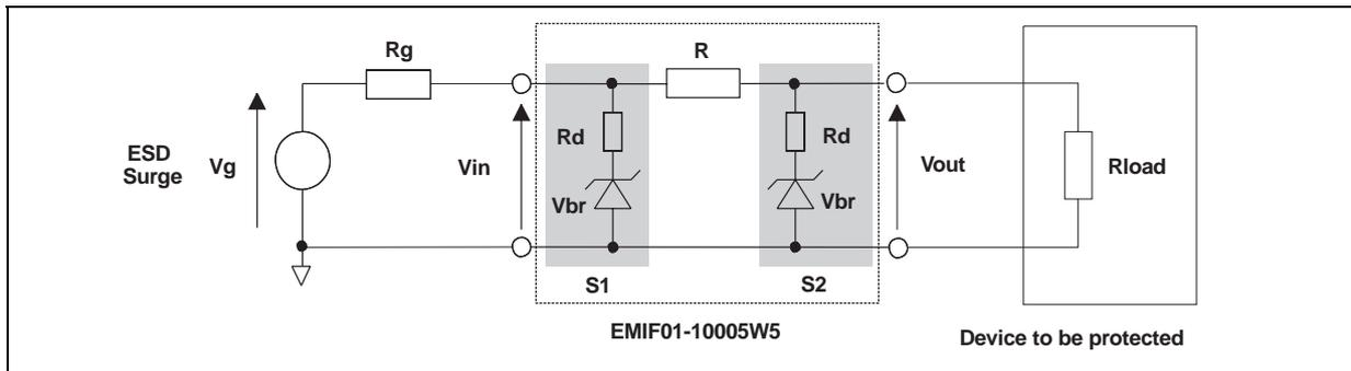
To have a good approximation of the remaining voltages at both Vin and Vout stages, we provide the typical dynamical resistance value Rd. By taking into account these following hypothesis :  $R \gg R_d$ ,  $R_G \gg R_d$  and  $R_{load} \gg R_d$ , it gives these formulas:
