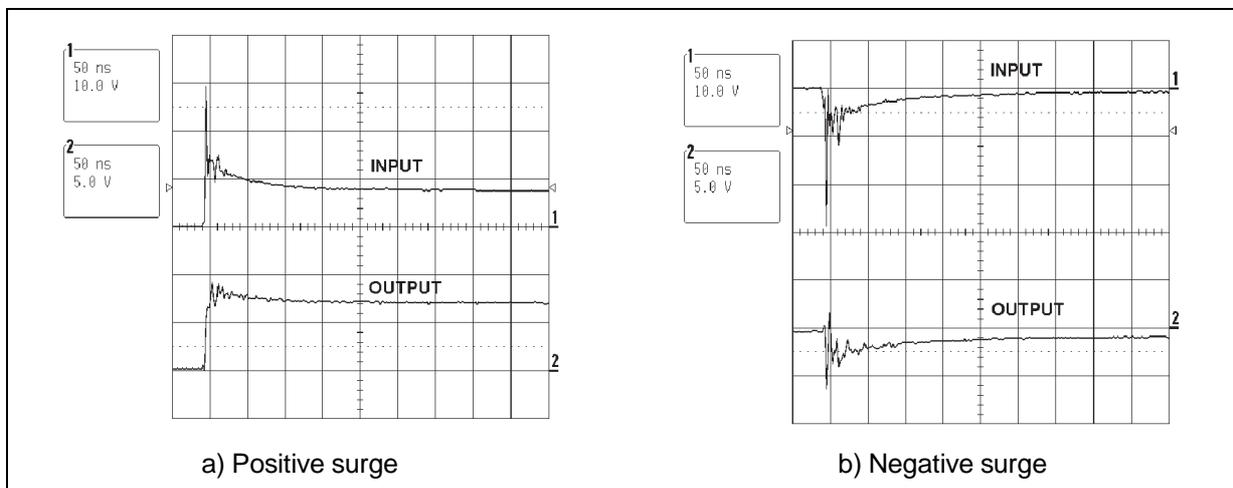
Please note that the EMIF01-10005W5 is not only acting for positive ESD surges but also for negative ones. For these kind of disturbances it clamps close to ground voltage as shown in Fig. A5b.
