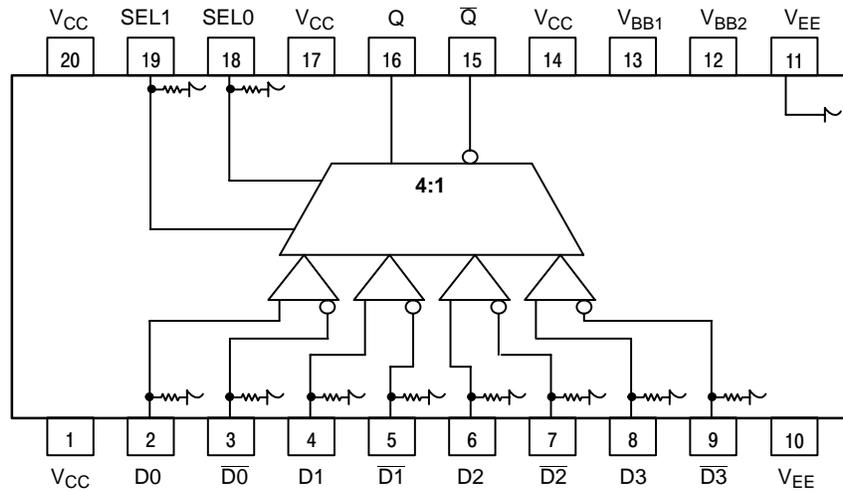
Warning: All  $V_{CC}$  and  $V_{EE}$  pins must be externally connected to Power Supply to guarantee proper operation.
