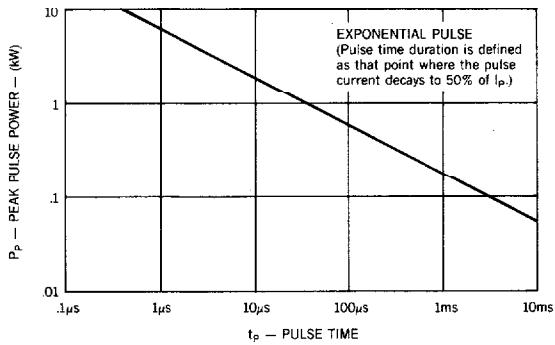
Figure 3. Derating Curve
