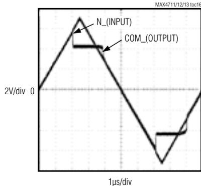
**FAULT TURN-ON DELAY AND RECOVERY TIME**
