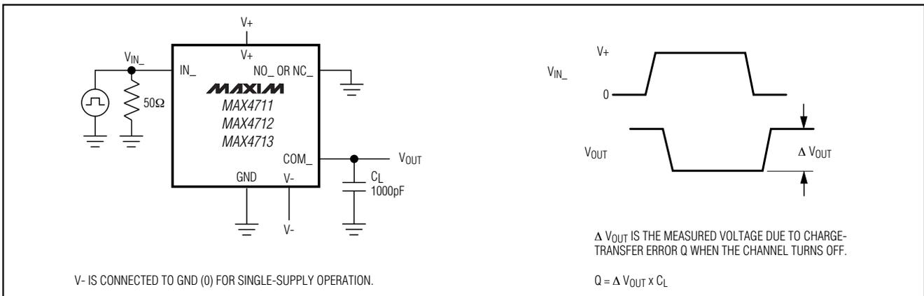
Figure 4. Charge Injection
