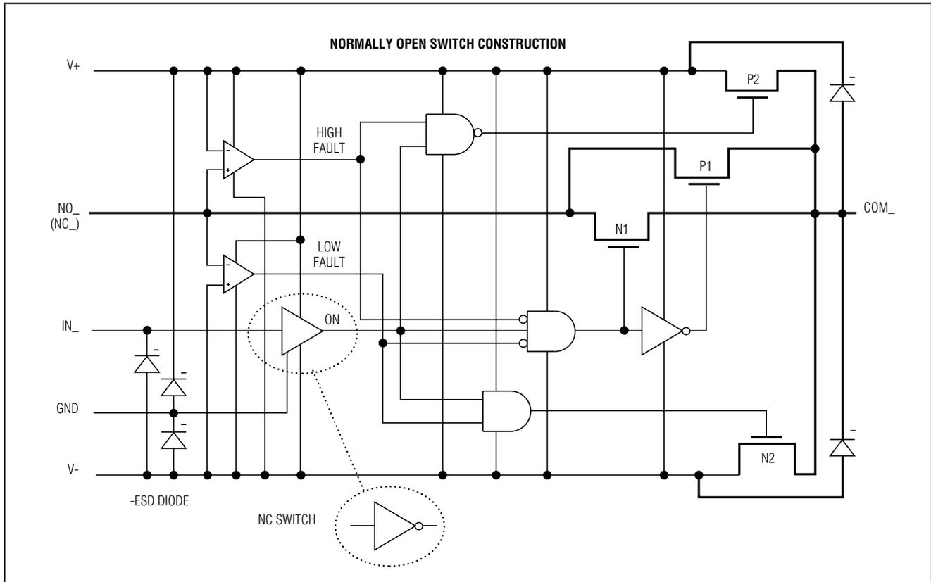
Figure 1. Block Diagram
