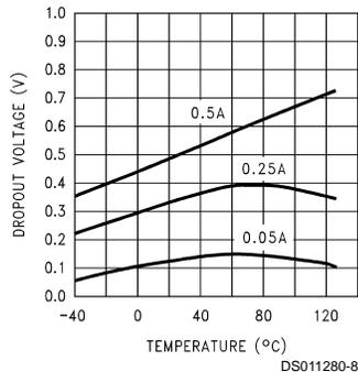
**Output Voltage vs Temperature**
