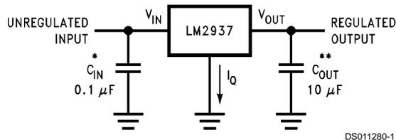
\* Required if the regulator is located more than 3 inches from the power supply filter capacitors.
