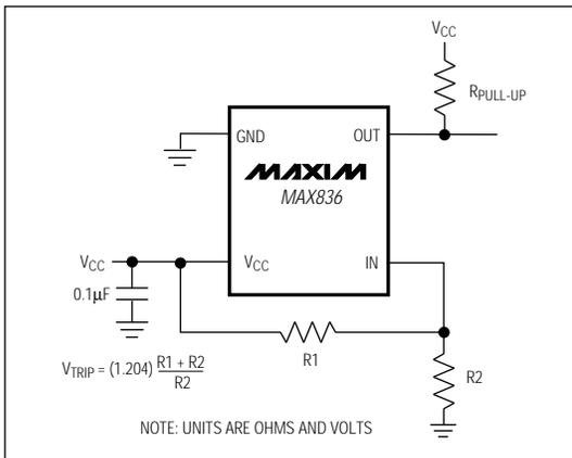
Figure 1. Programming the Trip Voltage, V<sub>TRIP</sub>
