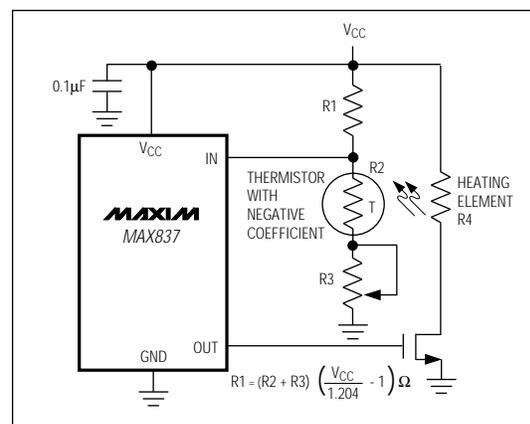
Figure 4. Heater Temperature Control
