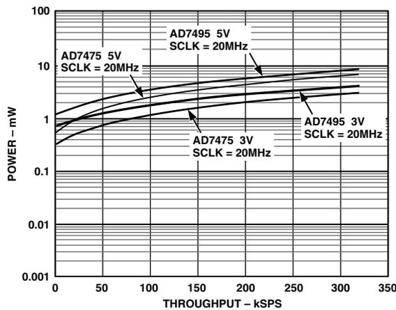
Figure 18. AD7495 Power vs. Throughput for Partial Power-Down
