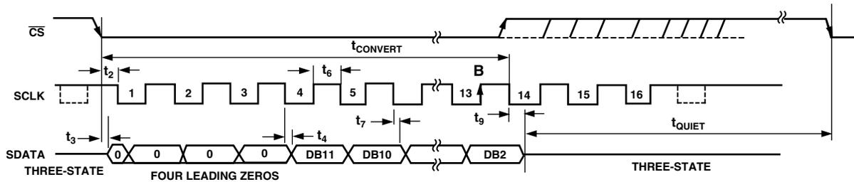
Figure 21. Serial Interface Timing Diagram – Conversion Termination
