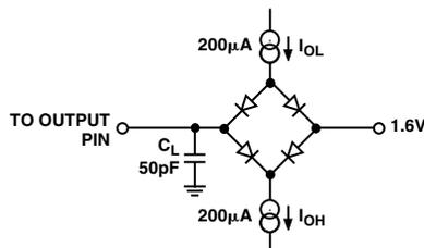
Figure 3. Load Circuit for Digital Output Timing Specifications
