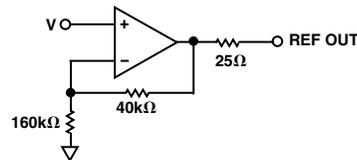
Figure 12. AD7495 Reference Circuit
