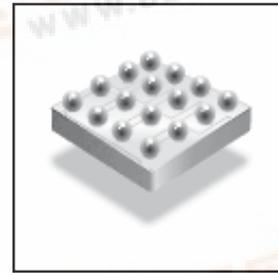
The FlipFET™ package, is one-third the footprint of a comparable SO-8 package and has a profile of less than .8mm. Combined with the low thermal resistance of the die level device, this makes the FlipFET™ the best device for applications where printed circuit board space is at a premium and in extremely thin application environments such as battery packs, cell phones and PCMCIA cards.
