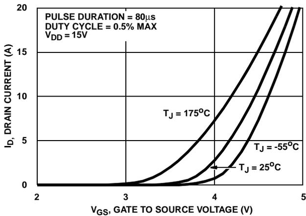
FIGURE 7. TRANSFER CHARACTERISTICS
