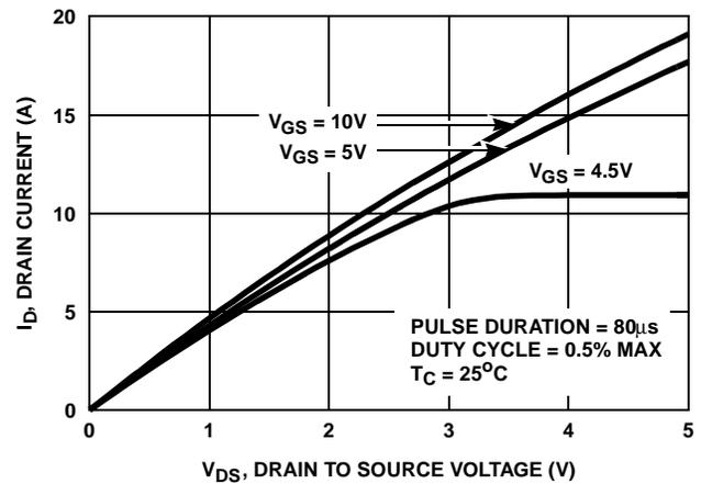
FIGURE 8. SATURATION CHARACTERISTICS
