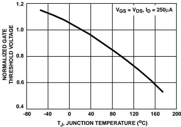
FIGURE 11. NORMALIZED GATE THRESHOLD VOLTAGE vs JUNCTION TEMPERATURE
