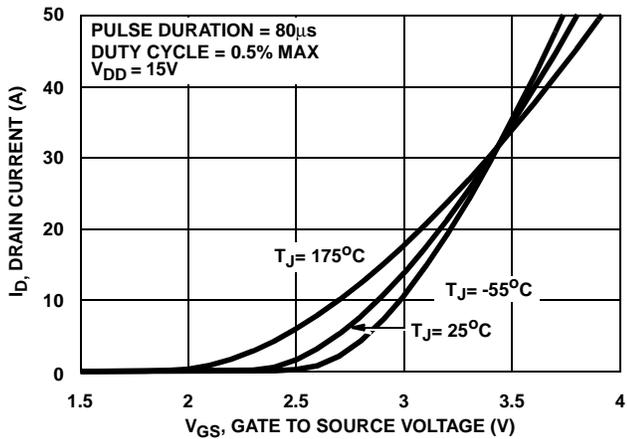
FIGURE 7. TRANSFER CHARACTERISTICS
