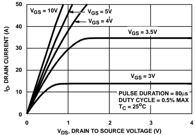
FIGURE 8. SATURATION CHARACTERISTICS
