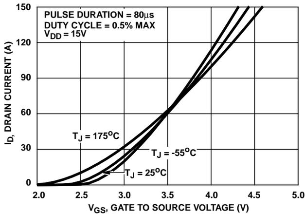
FIGURE 7. TRANSFER CHARACTERISTICS
