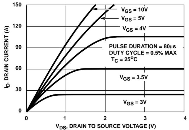
FIGURE 8. SATURATION CHARACTERISTICS
