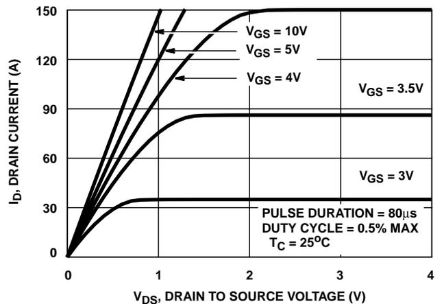
FIGURE 8. SATURATION CHARACTERISTICS
