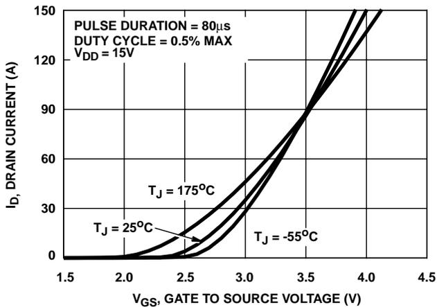
FIGURE 7. TRANSFER CHARACTERISTICS
