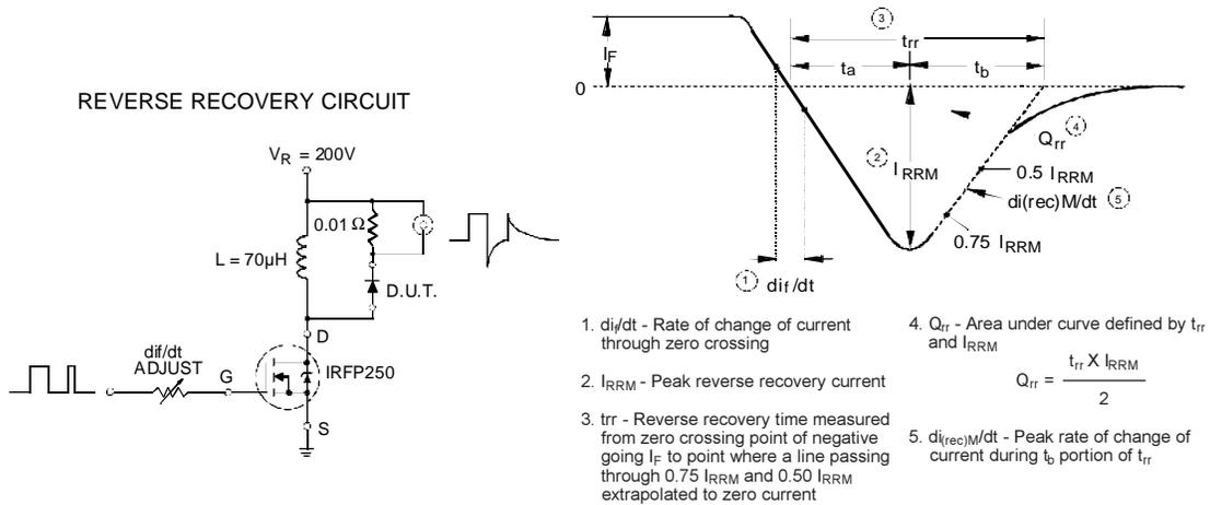
Fig. 9 - Reverse Recovery Parameter Test Circuit
