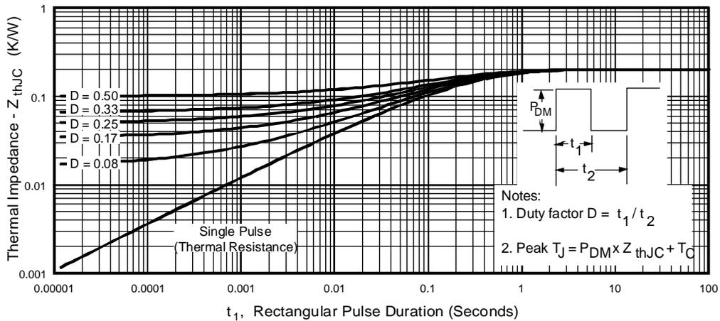
**Fig. 4** - Maximum Thermal Impedance  $Z_{thJC}$  Characteristics, (per Leg)
