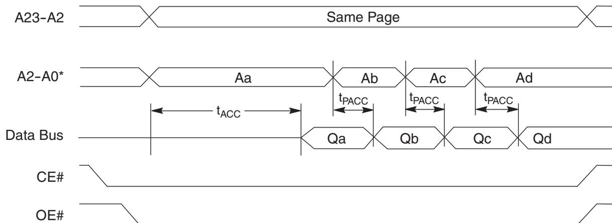
\* Figure shows word mode. Addresses are A2-A-1 for byte mode.
