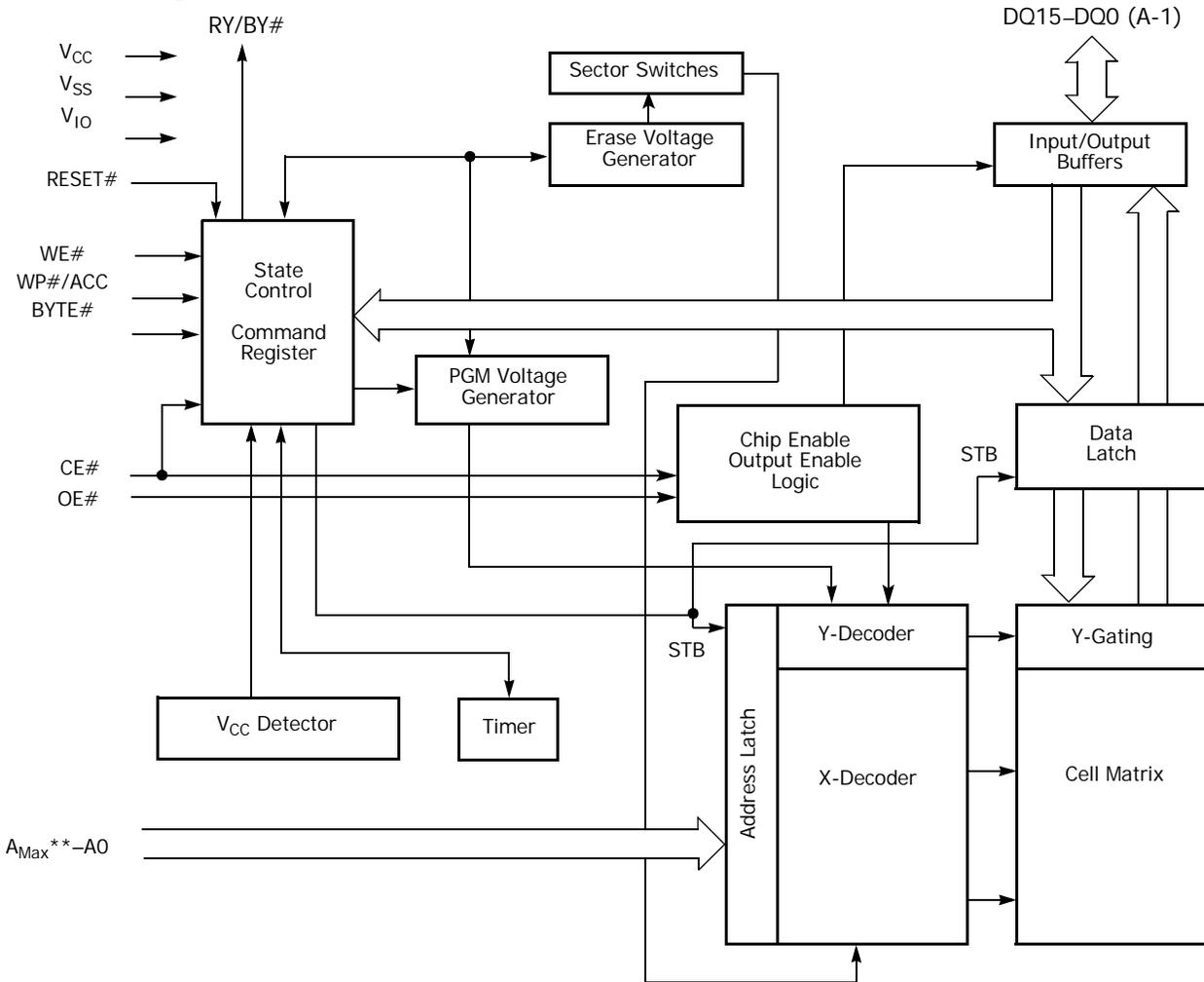
\*\*  $A_{Max}$  GL512N = A24,  $A_{Max}$  GL256N = A23,  $A_{Max}$  GL128N = A22
