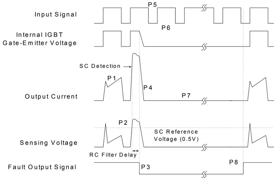
(with the external shunt resistance and CR connection)
