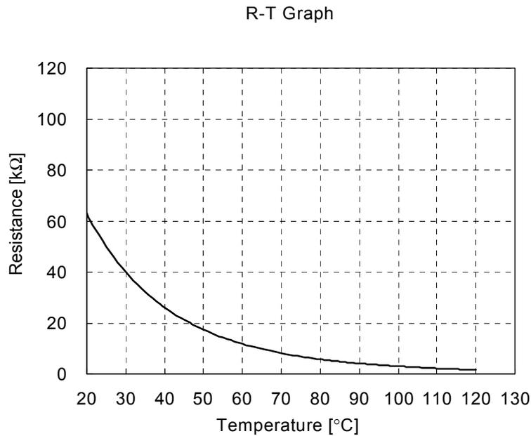
**Fig. 9. R-T Curve of the Built-in Thermistor**
