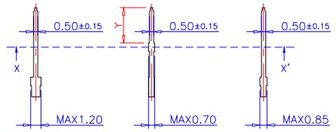
LEAD TYPE 1      LEAD TYPE 2      LEAD TYPE 3
