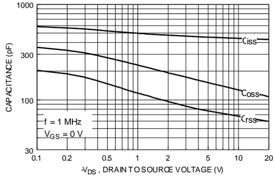
**Figure 8. Capacitance Characteristics.**
