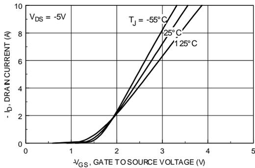
**Figure 5. Transfer Characteristics.**
