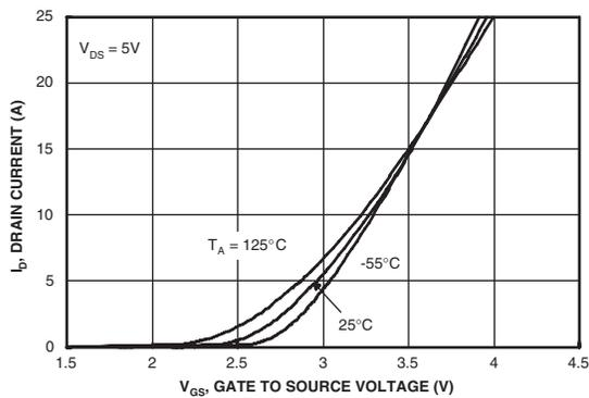
Figure 5. Transfer Characteristics.
