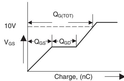
**Figure 15. Gate Charge Waveform**
