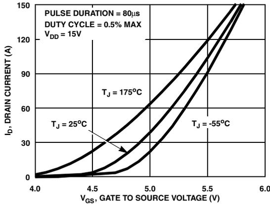
**Figure 7. Transfer Characteristics**
