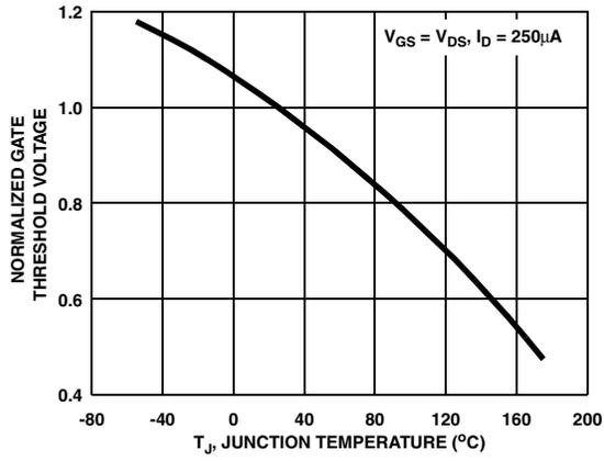
**Figure 11. Normalized Gate Threshold Voltage vs Junction Temperature**
