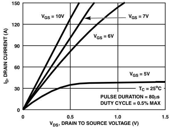
**Figure 8. Saturation Characteristics**
