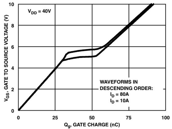
**Figure 14. Gate Charge Waveforms for Constant Gate Currents**
