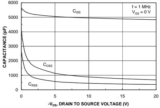
Figure 8. Capacitance Characteristics.
