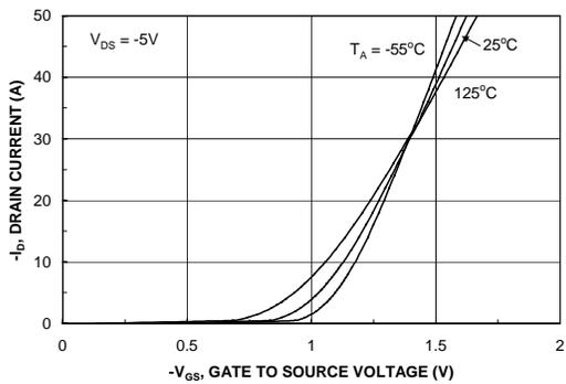
Figure 5. Transfer Characteristics.
