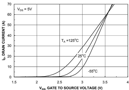
Figure 5. Transfer Characteristics.
