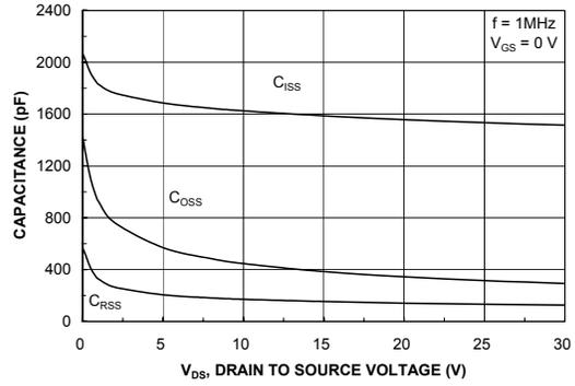
Figure 8. Capacitance Characteristics.
