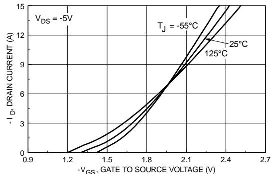
Figure 5. Transfer Characteristics.
