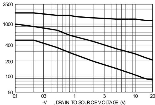
**Figure 8. Capacitance Characteristics.**
