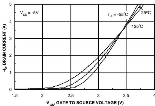
Figure 5. Transfer Characteristics.
