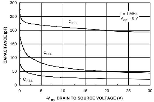
Figure 8. Capacitance Characteristics.
