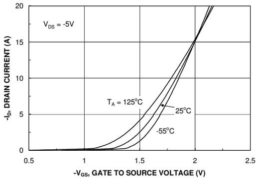
Figure 5. Transfer Characteristics.
