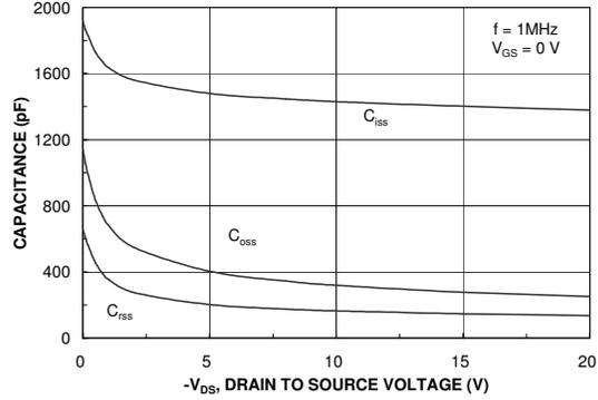
Figure 8. Capacitance Characteristics.
