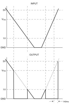
When operating properly with 5V in (for example),  $V_{OUT}$  will also be about 5V. When  $V_{IN}$  starts to fall,  $V_{OUT}$  will follow it down as shown. When  $V_{IN}$  drops below  $V_{TH}$ ,  $V_{OUT}$  drops to ground ("issues a RESET") and stays there unless  $V_{IN}$  also falls below its minimum operating voltage, approx. 1V. At this point, the supervisor loses control, and its output may rise, only to again follow  $V_{IN}$  down to the ground.
