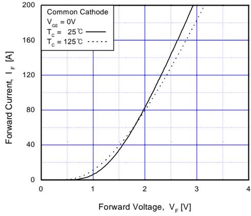
Fig 19. Forward Characteristics
