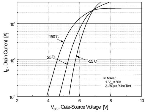
Figure 2. Transfer Characteristics
