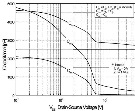
Figure 5. Capacitance Characteristics
