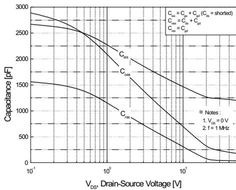
Figure 5. Capacitance Characteristics
