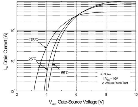
Figure 2. Transfer Characteristics
