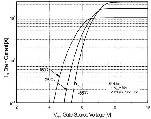
Figure 2. Transfer Characteristics
