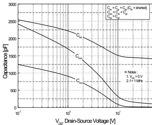
Figure 5. Capacitance Characteristics
