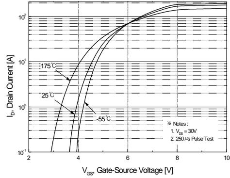
Figure 2. Transfer Characteristics
